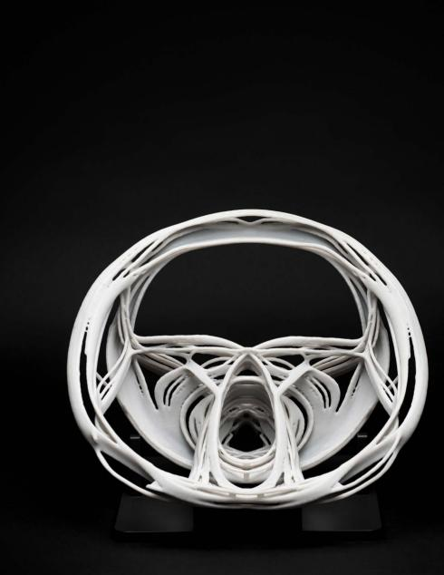
Three 3D printed results of steering wheel design process case study, named after the generative system used: Heterogenous HoneyComb (page 29), Delaunay Construction (page 30) and Custom Stress Lines (page 33).
